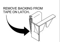
MOUNT LATCH TO DOOR BY PLACING IT IN THE NOTCH IN THE TOP OF THE TEMPLATE AS ILLUSTRATED. PRESS IN PLACE.
